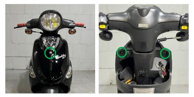
2) Once the screws have been removed, carefully remove the front panel, granting access to the wiring and existing 12V power outlet.
